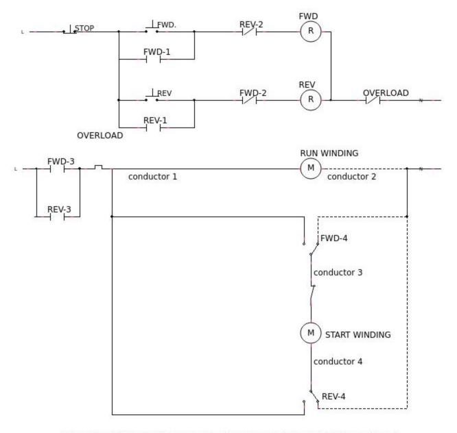
NOTE: THIS MOTOR MUST COME TO A COMPLETE STOP BEFORE BEING REVERSED 4 CONDUCTORS PLUS A GROUND ARE REQUIRED BETWEEN MOTOR AND RELAYS
